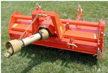
The reverse rotation of our tiller tines forces the tiller down into the ground for deep smooth cultivation while bringing debris up over the top of the rotor. This unique action deposites larger debris first then covers it with finely pulverized soil particles for a smoother cleaner finish. Got the final results
