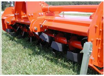
T20 Series Rotary Tillers from Phoenix Line assure you years of trouble free performance even under the most demanding applications. The load bearing frame on which the protective hood and transmission are mounted make this machine extremely sturdy. The unique design dramatically reduces the possibility of clogging, even in sticky or wet soil conditions.
