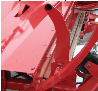
Figure 6.2 Adjusting the bale guides
