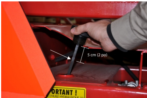
Figure 5 – Oil in Hydraulic oil tank
