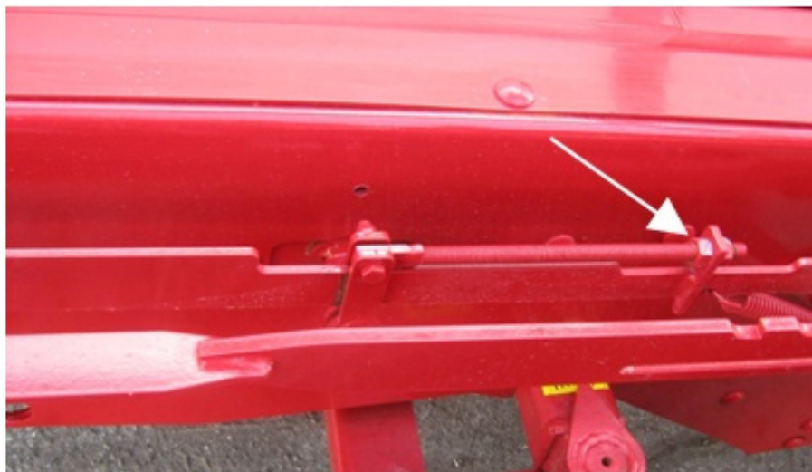
Figure 43 – Adjusting the pusher trigger (nuts)
