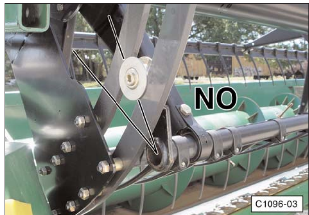
Incorrect orientation (roller is above or following tine tube into header).
